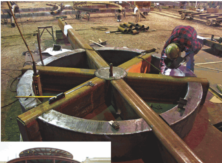
The winter garden atrium's central connection ring (above) was shop fabricated.
